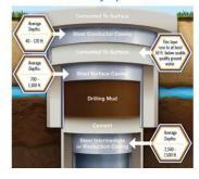
A drilling rig begins the underground construction process by installing steel pipe and cement (surface casing) to protect groundwater. Surface casing is set at least 50' below the aquifer, which is typically about 1,000' below the surface.
