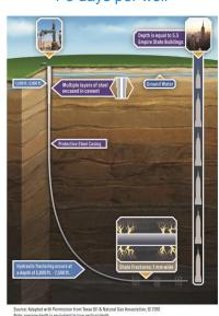
A production rig arrives and drills to a depth of 7,000 to 8,000 feet. The horizontal portion of the wellbore can extend more than two miles.
