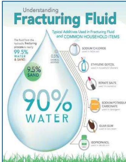
**Hydraulic Fracturing:** A safe, highly engineered technology developed in the 1940s. Fluid is pumped over a mile below the earth's surface under pressure to create hairline fractures in the rocks.
