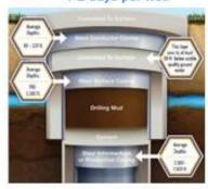
A drilling rig begins the underground construction process by installing steel pipe and cement (surface casing) to protect groundwater. Surface casing is set at least 50 feet below the aquifer, which is typically about 1,000 feet below the surface.
