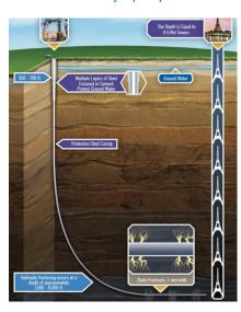
A production rig arrives and drills to a depth of 7,000 to 8,000 feet. The horizontal portion of the wellbore can extend more than two miles.
