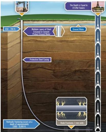
A production rig arrives and drills to a depth of 7,000 to 8,000 feet. The horizontal portion of the wellbore can extend more than two miles.
