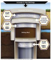
A drilling rig begins the underground construction process by installing steel pipe and cement (surface casing) to protect groundwater. Surface casing is set at least 50' below the aquifer, which is typically about 1,000' below the surface.
