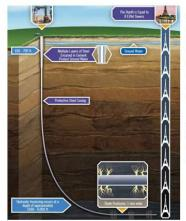
A production rig arrives and drills to a depth of 7,000 to 8,000 feet. The horizontal portion of the wellbore can extend more than two miles.
