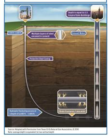
A production rig arrives and drills vertically to a depth of 7,000 to 8,000 feet. From this depth, the horizontal portion of the wellbore can extend more than two miles. Additional layers of protective steel casing and cement are installed. Well Completions (6-9 days per well)
