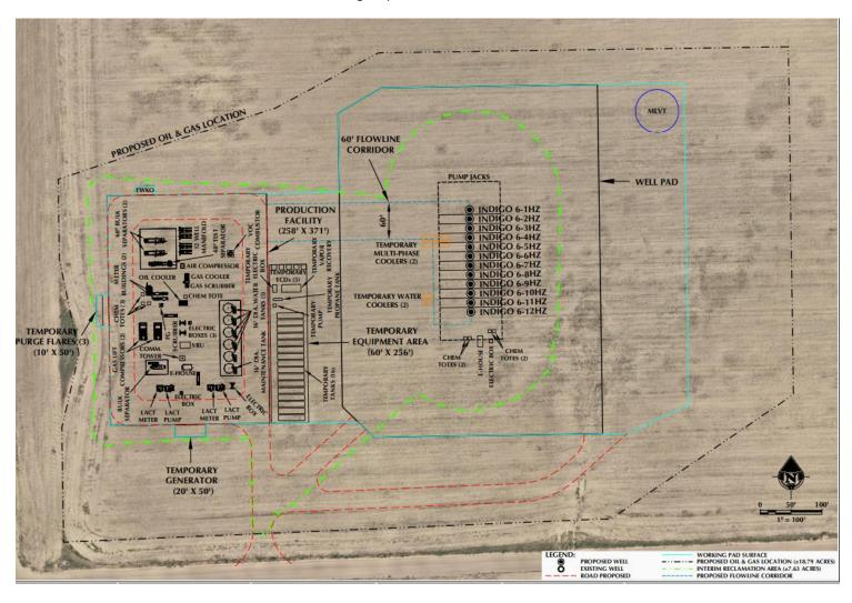
This proposed site layout is shown above. All 12 of the wells drilled from the surface location and running west.
