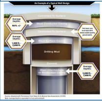
A drilling rig begins the underground construction process by installing steel pipe and cement (surface casing) to protect groundwater. Surface casing is set at least 50' below the aquifer, typically about 1,5000'+ below the surface.
